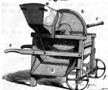
THE DISC TURNIP-SLICER FOR SHEEP.
